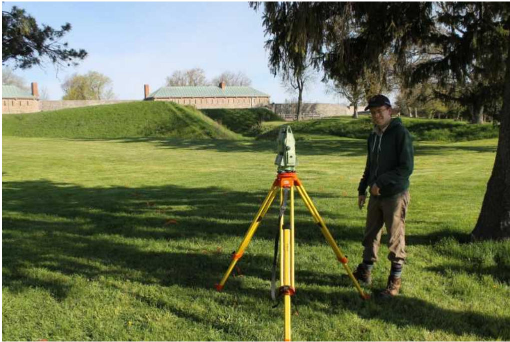
Figure 8 Teaching Assistant Owen Harvey setting up grid with Total Station. View facing north with ravelin and barracks in background.
