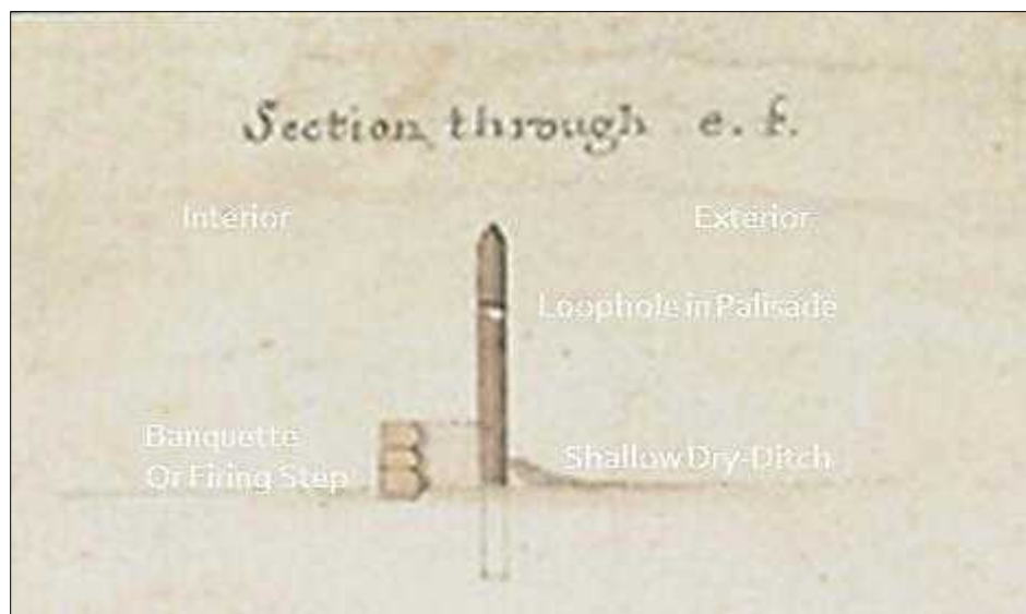
Figure 50. Detail of Plan of Fort Erie, Built under the Direction of John Montessor, Engineer, 1764 . By Francis Pfister, 1766 showing details of perimeter.
