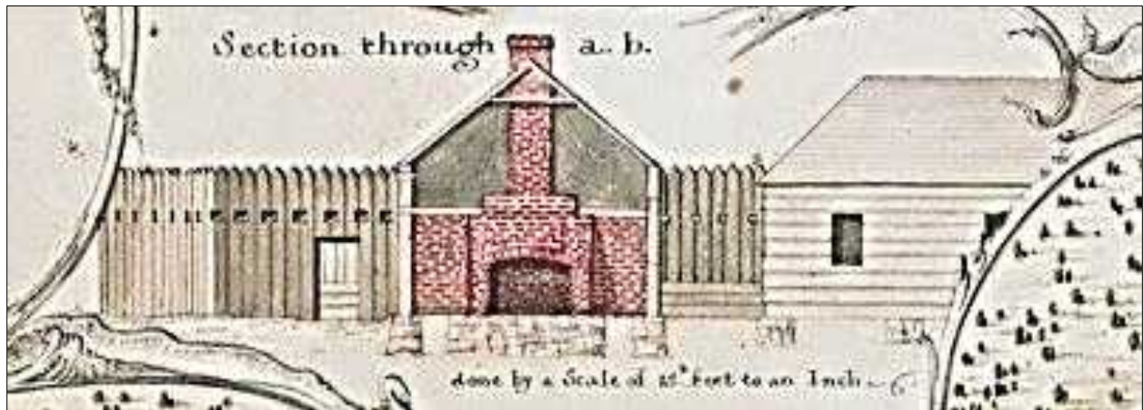
Figure 48. Detail of Plan of Fort Erie, Built under the Direction of John Montrossor, Engineer, 1764 . By Francis Pfister, 1766 showing cross-section with stockade/palisade, sally port, stone piers, brick fireplace and chimney, and squared timber construction.
