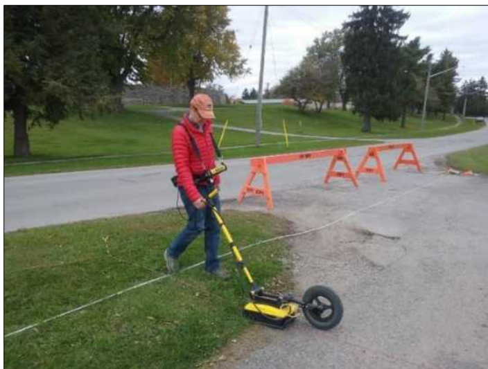
Figure 8. The GPR survey used a tow wheel to log data below the asphalt.
