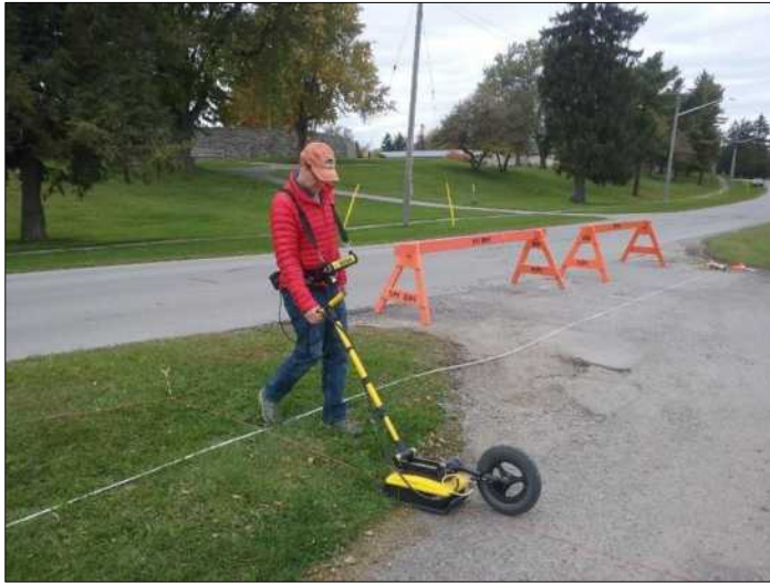
Figure 12. The Sensors and Software Noggin ground-penetrating radar system used in the survey of the lakeshore
