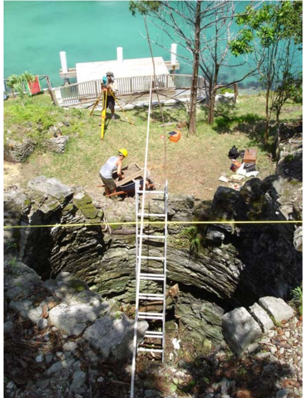
Figure 8 Recording the lime kiln from inside and out using the total station and tapes strung across the charge hole. The kiln floor is about 5 metres below the tapes.
